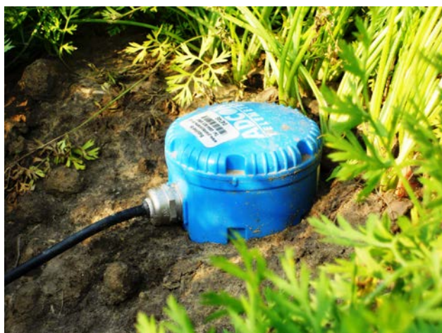
Figure 2: Soil moisture sensor showing insertion into carrot bed alongside rows
