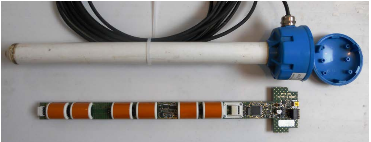
Figure 3: Soil moisture sensor showing internal construction
